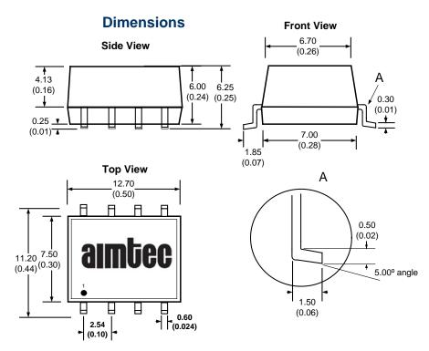
All dimensions are in mm (inch) All Pins are on a 2.54mm (0.10inch) pitch with tolerance of  $\pm 0.25$ mm (0.01inch)
